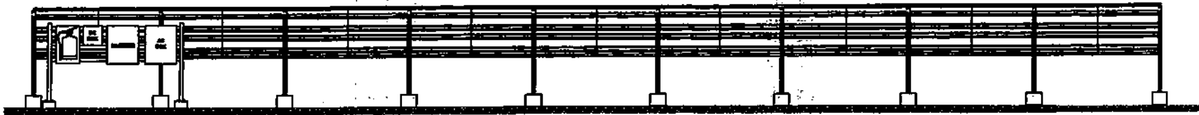
REAR ELEVATION WITH FIRE EXTINGUISHER, DC BOX, INVERTER & AC BOX CalSPV-BDC-17.011 SCALE NTS
